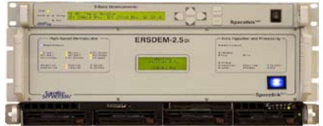
ERSDEM-2.5 Dii with S-Band down-converter, demodulator and integrated Raw Data Ingestion platform and data processor for Real-time level-0 processing and simulation
